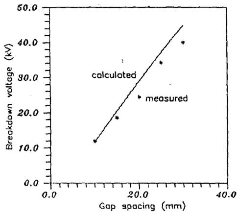
Fig.3 BDV in different gap spacing under ac voltage
