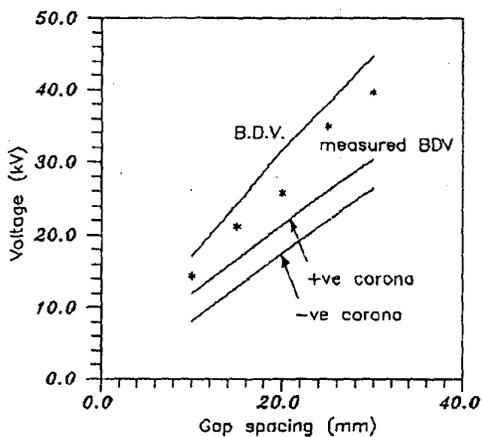
Fig.5 Effect of gap spacing on corona onset and BDV With 2 kV dc biasing voltage.
