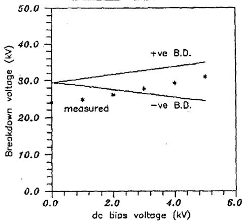
Fig.4 Effect of dc biasing voltage on BDV with fixed particle contamination
