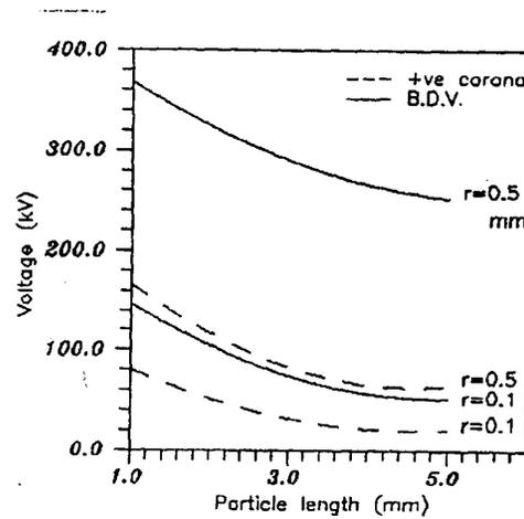
Fig.7 Effect of particle dimensions on corona onset and BDV with 5 kV dc biasing voltage for SF<sub>6</sub>
