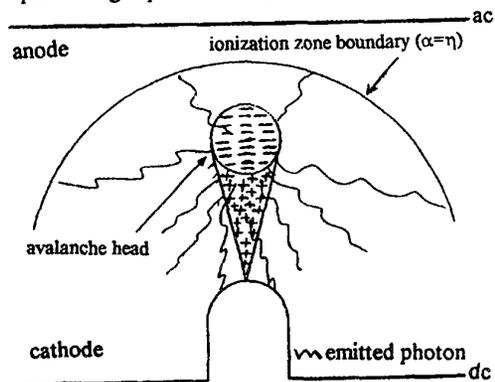
Fig.2 Growth of the primary avalanche and Emission of photons in negative corona.
