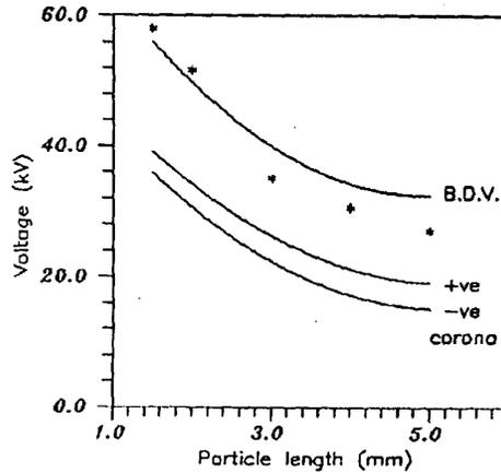
Fig.6 The BDV versus particle length under dc/ac Voltage
